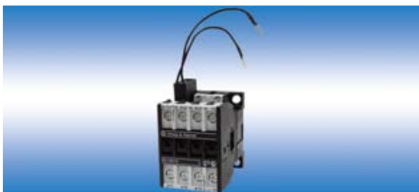
RC- Units protect the contactor coils against voltage peaks & harmonic waves.
